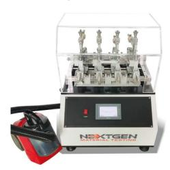
to determine the rating of abrasion. This unit conforms ASTM and ISO methods as well as the LP-463KB-06-01 commonly referred to as the Chrysler, FCA and Stellantis method. Learn more about the <a href="Certified Wyzenbeek Abrasion Testing System and Testing Procedures">Certified Wyzenbeek Abrasion Testing System and Testing Procedures</a>.
