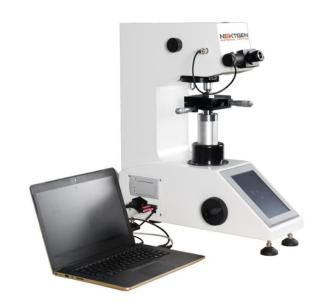
**AGEN** - Analogue Micro Vickers and Knoop Hardness tester measurements are made through the eyepiece. The operator must first
