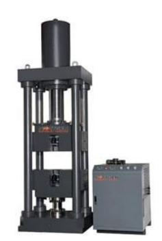
Clearance-free structure and actuator up and down to adjust the test space offers easy operation and high efficiency. This machine is mainly used for tensile test of metallic materials. It provides closed loop control of constant force, constant displacement and constant extension, smoothly switching among them.
