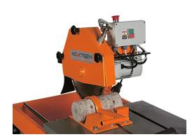
The NG-CoreTrim 600 - Rock Core Cutter and Masonry Saw: Engineered as a Universal Cutting solution, it precisely cuts hardened concrete, rock, and natural stone test specimens to the required sizes for testing. 600mm diameter blade with 250mm cutting depth and 500mm maximum cutting stroke.
