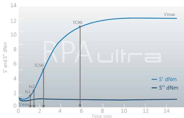
The isothermal cure tests on rubber compounds are among the most common and essential studies done. The BareissOne software determines all significant test parameters, including maximum and lowest torque, TC values, reaction time and rate, etc., and makes them available to the user in tabular or/and graphical form for additional analysis.
