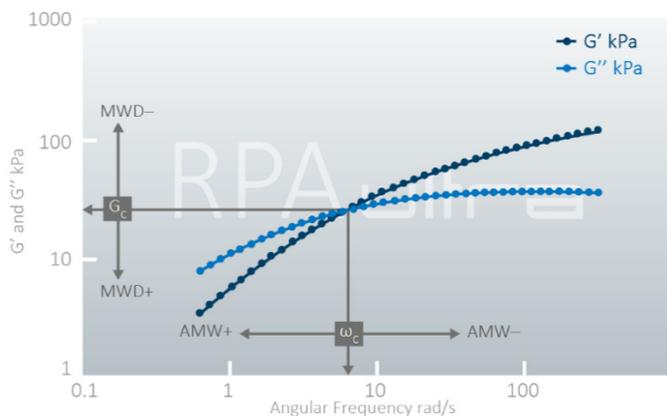
The user thoroughly follows the viscoelastic behavior and molecular structure by analyzing a sample over a broad range of frequencies (molecular weight and molecular weight distribution). Moreover, due to the sample's frequency-dependent behavior, several viscoelastic parameters, including complex modulus, elastic modulus, loss modulus, complex viscosity, phase angle, etc., are calculated at each frequency.
