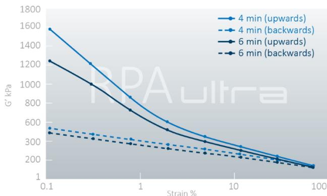
A specimen's behavior can be seen when it is measured over a broad strain range, such as the linear viscoelastic range (LVE) up to large amplitude oscillatory shear (LAOS). The Payne test, used to analyze the (filler/polymer) filler networks at low strain amplitudes, provides the details on the filler content and filler dispersion levels.
