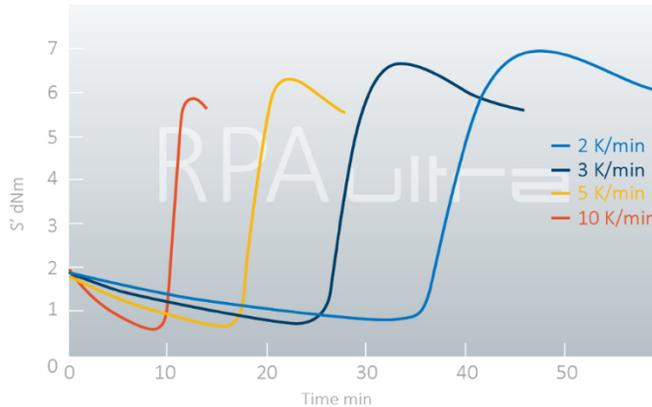
Non-isothermal measurements (temperature sweep) are frequently performed at various heating rates to assess a sample's behavior over a wide temperature range. The BareissOne program includes a module for kinetic calculations made possible by this measurement at various heating rates.
