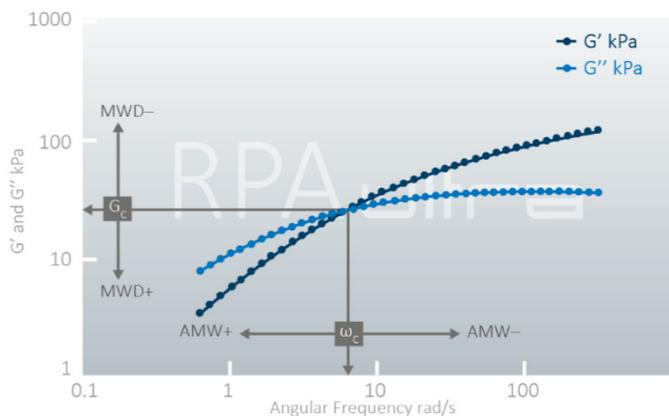
The user thoroughly follows the viscoelastic behavior and molecular structure by analyzing a sample over a broad range of frequencies (molecular weight and molecular weight distribution). Moreover, due to the sample's frequency-dependent behavior, several viscoelastic parameters, including complex modulus, elastic modulus, loss modulus, complex viscosity, phase angle, etc., are calculated at each frequency.
