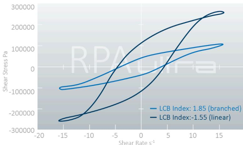
LAOS is a strain sweep used to examine and assess a sample's nonlinear viscoelastic behaviour at relatively large amplitudes.
