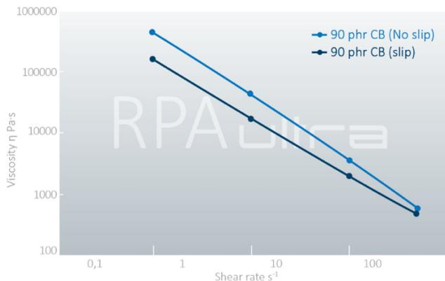
The problem of Wall Slip is a severe obstacle in producing rubber compounds.
