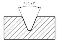
Radius of notch base  $r_{\rm N} = 0.25 \text{ mm} \pm 0.05 \text{ mm}$
