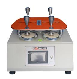
accuracy of abrasion strength is determined by the specific number of cycles conducted until a hole appears in the test area of the fabric specimen. This unit is the industry leader for Certified Martindale Abrasion Resistance Testing designed to produce accurate, repeatable and user-friendly testing results every time.
