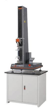
• Servo motor with precise planet-gear speed reducer provides higher driving efficiency, low noise and free of maintenance. Because there is no need to replace lubricants the system's work life is prolonged.
