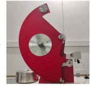
The GenElm Series comes with a simple touch-screen interface, automatic specimen cutting, and pneumatic clamping for stable handling of samples. Different pendulum options allow the user to cover several testing ranges, while the built-in system collects and processes the data. This combination of functions makes the instrument practical for everyday laboratory work and a reliable solution for routine testing.
