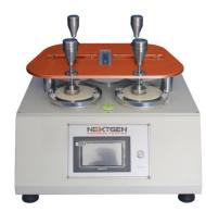
GenDale is mainly used to test shoe fabric, shoe lining, and many other types of shoe related materials. The unit can test up to four specimens at the same time for abrasion. The fabric specimen is measured by having rubbing applied on it via a complex direction of back and forth motion. The accuracy of abrasion strength is deter- mined by the specific number of cycles conducted until a hole appears in the test area of the fabric specimen.
