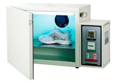
The UV discoloration meter is a machine is used to simulate an environment of sunlight radiation on a specimen to identify the resistance of fabric to discoloration. NextGen offers two primary models based on size and temperature regulations to help meet your ASTM standards.
