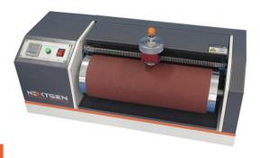
GenDin, is designed to conform to the ASTM D5963 and ISO 4649 standards. This top quality and highly popular abrasion tester will allow you to measure the abrasion resistance of rubbers (vulcanized thermo set rubbers and thermoplastic elastomers) that are subject to abrasive/frictional wear on their actual service. Since wear is always a result of abrasion, different test methods have been developed for the simulation of long-term wear.
