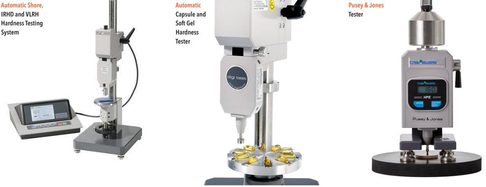
Digi Test II is an automatic Shore, IRHD and VLRH hardness testing system. The unit comes equipment with 4 main components: Electronic unit, the loading module (pick-up bracket), the test stand, and the interchangeable measuring unit for methods of Shore, IRHD and VLRH. The unit complies with DIN ISO 7619, DIN ISO 48, DIN EN ISO 868, NF EN ISO 868, ASTM D 2240, BS 903 Part. A 26, NFT 46-003, ASTM D1415, DIN ISO 27588 standards.
