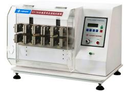
GenFlex tests the ability of rubber products to withstand repeated flexing without developing cracks is of prime importance where such products are used in conditions undergoing repeated flexing.
