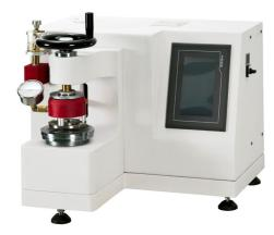
GenBurst is designed to test anti-rupture strength of variety of materi- als such as leather, paper and fabric. The unit tests the resistance of specimens to bursting using a hydraulic diaphragm bursting tester.
