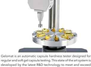
regular and soft gel capsule testing. This state of the art system is developed by the latest R&D technology to meet and exceed the highest quality standards for gelatin capsule testing. The system comes standard with your desired testing head and can be upgraded to optional accessories for maximum efficiency.
