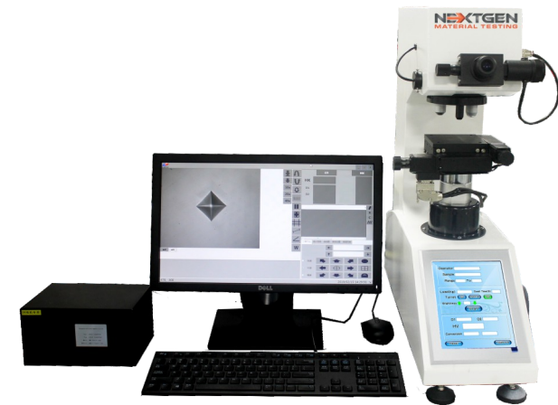
NEXTGEN MICRO VICKERS/KNOOP HARDNESS TESTER
