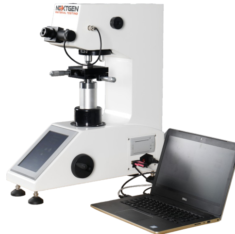
NEXTGEN MACRO VICKERS HARDNESS TESTER
