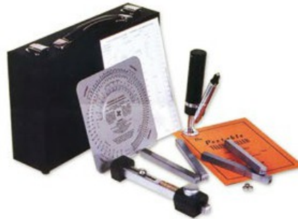
NEXTGEN TELEBRINELLER BRINELL HARDNESS TESTING SYSTEM
