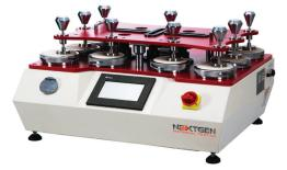
GenDale is mainly used to test shoe fabric, shoe lining, and many other types of shoe related materials. The unit can test up to four specimens at the same time for abrasion. The fabric specimen is measured by having rubbing applied on it via a complex direction of back and forth motion. The accuracy of abrasion strength is determined by the specific number of cycles conducted until a hole appears in the test area of the fabric specimen.
